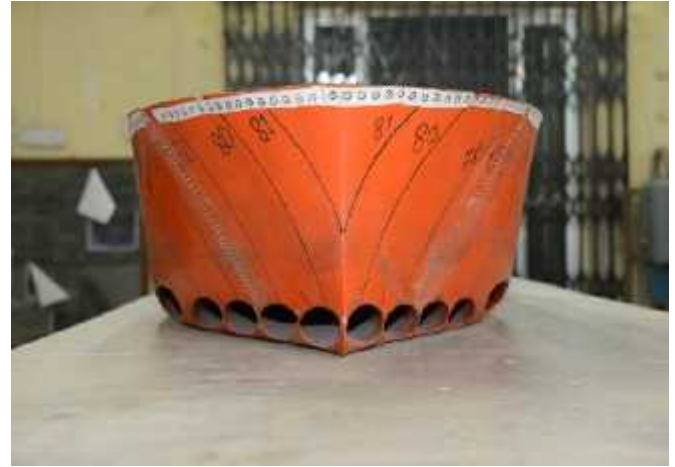
Figure 3: Model of Ballast Free Ship
