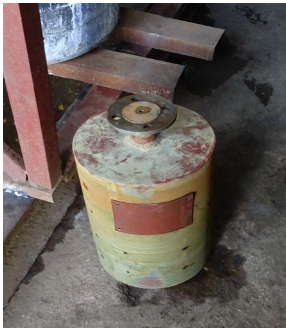
Figure 6: Central rotor of the drum test apparatus with the attached test plate
