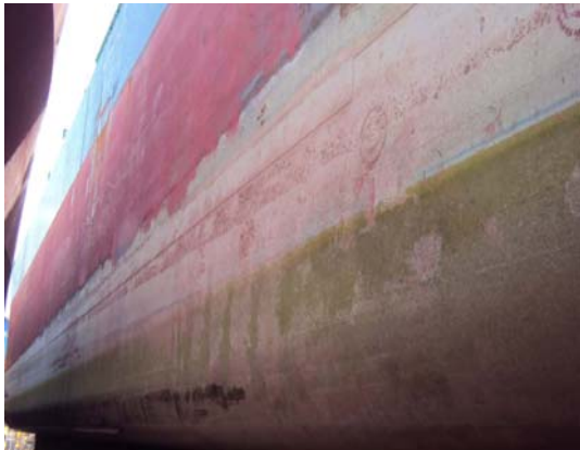
Figure 2: Photographs of a vessel taken on arrival at dry-dock indicating areas on antifouling paint deterioration
